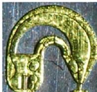
**Figure 2. A typical unwanted Parallel-Flow pattern where the denser phase remains close to the wall**
