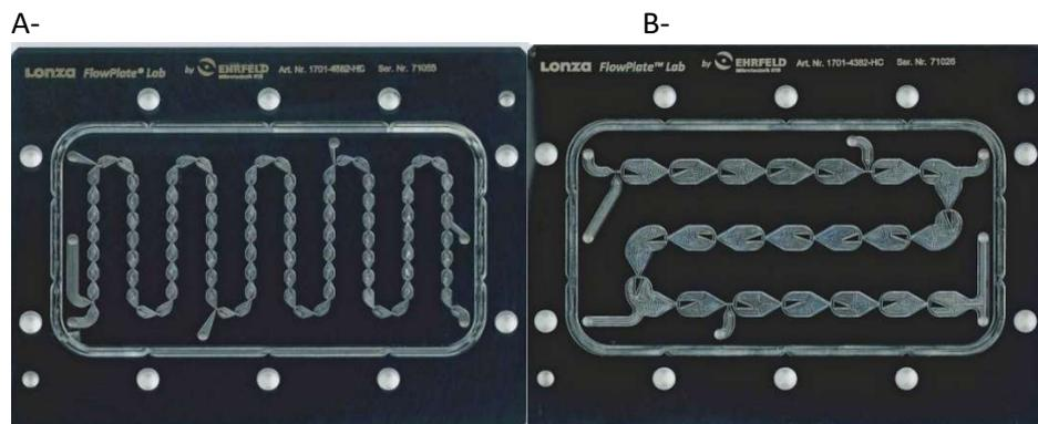
Figure 3. FlowPlate® Lab with LL-Triangle-Structure for small flow rate applications (A– 1–15 mL/min) and a scalable version at ten times this basic flow rate (B– 15-150 mL/min)
