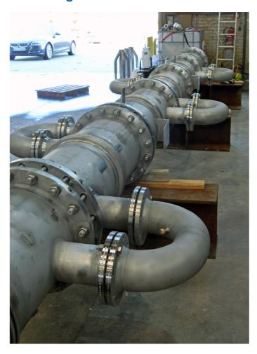
Ehrfeld Mikrotechnik BTS designed, manufactured and supplied a MIPROWA® production reactor for Shaoxing Eastlake Biochemical (China) with a production capacity of up to 10,000 t/a. The company serves the agrochemical global market segment with the production of active ingredients. The production plant in Shaoxing was launched successfully in mid-September 2016. The MIPROWA® technology is using millistructures on a production scale. Same channel geometries
